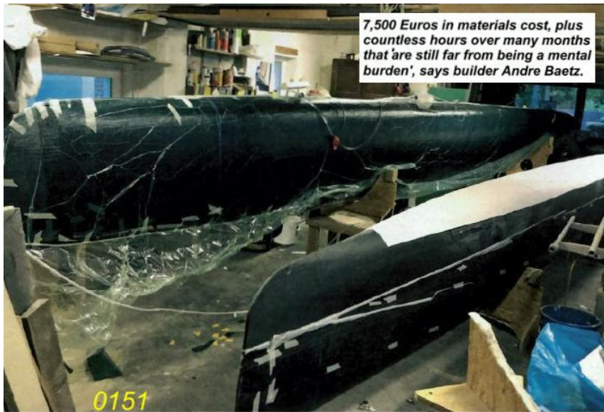
In the heated workshop with direct access to the living room, Baetz built the two floats, C-Foils, daggerboard and rudder blade, using CF and the vacuum infusion process
